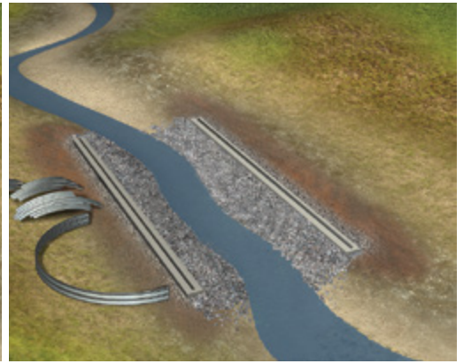
The first arch segment is completely assembled on the ground.
