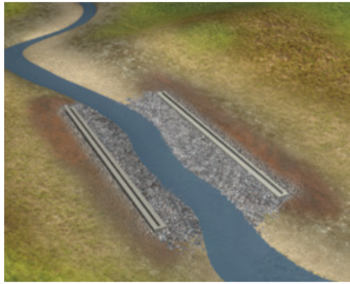
Precast or cast-in-place concrete footings are set over the prepared site.
